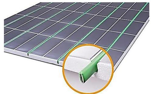
*The pressure-resistant, 20mm-strong heating element including pre-installed thermal conductivity panels of aluminium and a lower thermal insulation. The electrical, self-regulating heating tape lies in proper form within the oval channel.*
